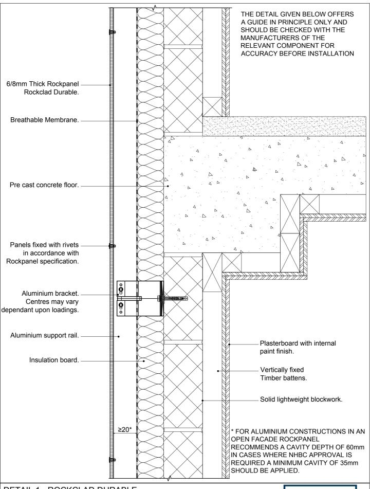
DETAIL 1 - ROCKCLAD DURABLE VERTICAL SECTION ALUMINIUM SUBSTRUCTURE TO STRUCTURAL CONCRETE & LIGHTWEIGHT BLOCKWORK.
